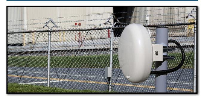
The **Radon MRS** detector is a linear barrier based on X-band microwave technology. It comprises a transmitter and a receiver unit, which create a perimeter protection with coverage up to 300 m. It is very simple to install, but it has high security performances. The microwave signal is digitally converted and analyzed by a microprocessor with an efficient and innovative algorithm.
